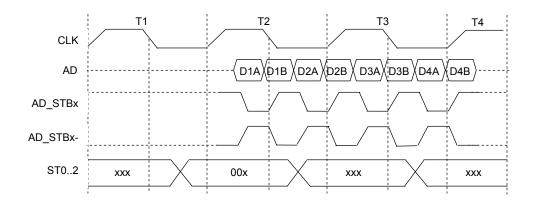
Compaq Evo and Workstation Personal Computers4-13 Featuring the Intel Pentium 4 Processor Figure 4-7. AGP 4X Data Transfer (Peak Transfer Rate: 1064 MB/s)
